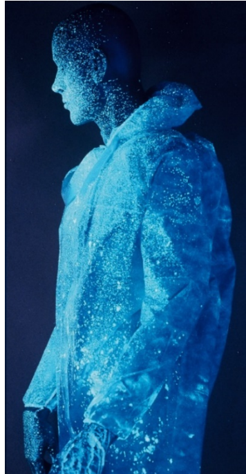
Figure 5.5 MWF droplet deposition from the use of compressed air.
