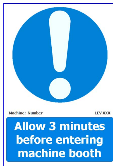
Figure 4.4 Safety labelling for the door of a CNC enclosure.
