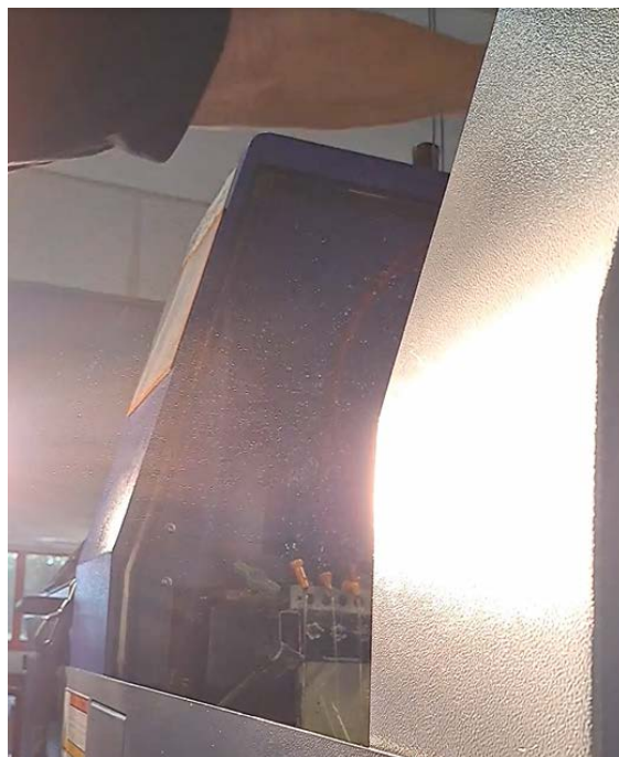
Figure 4.2 Photo showing visualisation of mist using a dust lamp.
